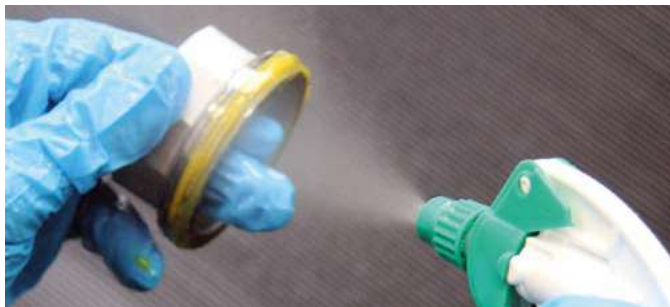
Removing sealant with GS 200
