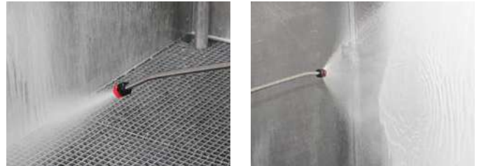
Applying cleaner with compressed-air foam lance
