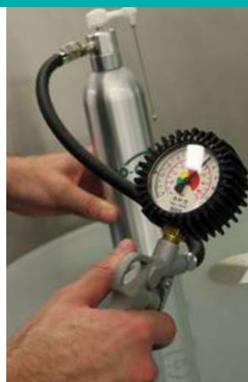
Unscrew bottle – fill in cleaner – screw down – top up with compressed air
