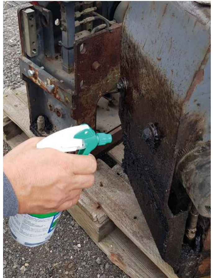
Removing bitumen with GS 200
