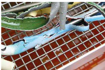
Paint removal in an ultrasonic bath with Poly Strip 100
